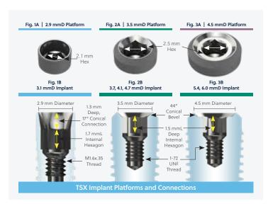
implant platform into the internal hex of the implant. The internal hex configuration is 2.5 mmD flat-to-flat with a depth of 1.5 mm. Below the hexagon is a continuation of the inner chamber which leads into the threaded area where the appropriate fixation screw with 1–72 UNF thread is received.
