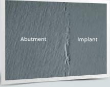
**Friction-Fit Technology** SEM at 150X magnification displays the mechanical interlock in the hexagonal engagement area between the flats of the implant and abutment.
