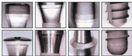
Fig. 3. SEM Examination: SwissPlus implants with (top, left to right): (1) surgical cover screw (2 mm long); (2) fixture mount/transfer/abutment; (3) straight abutment; and (4) threaded apical end. ITI synOcta with (bottom, left to right): (1) cover screw; (2) SwissPlus fixture mount/transfer/abutment; (3) ITI solid abutment; and (4) unthreaded apex.
